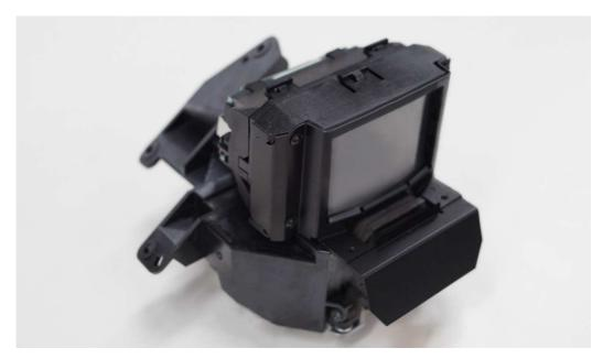
Automotive HUD projection unit using laser scanning technology
