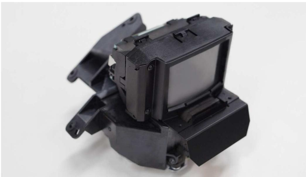
Automotive HUD projection unit using laser scanning technology
