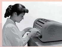
The Ricopy 101, Japan's first desktop diazo-wet copier to integrate exposure and development (1955)
