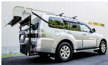
Vehicle fitted with road surface inspection system
