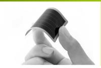
Advanced film-based, lightweight solar cells that can generate electricity in indoor lighting or in shade
