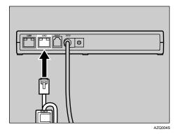
Connect the other end of the cable to network devices, such as HUB, etc.
