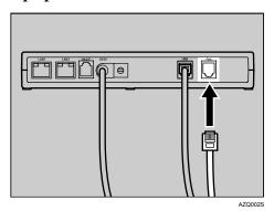
**1** Connect the other end of the white telephone line cable to the LINE port of the facsimile.
