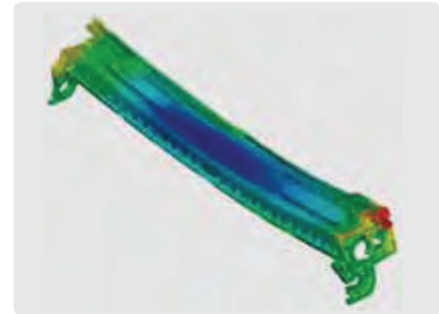
Analysis of deformation after unmolding
