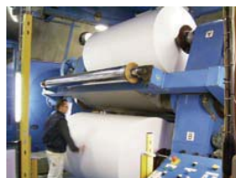
Automatic refilling process to transfer a 200-cm-wide roll paper to another rolling conveyor. The optimized operational timing prevents paper out caused by failed refilling.
