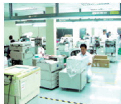
Manufacturing recycled copiers at Ricoh (Thailand) Ltd.
