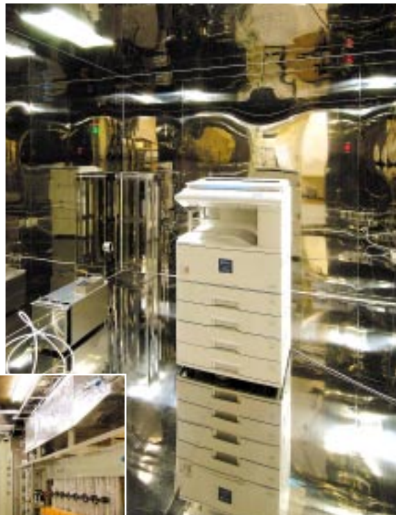
Emission-measuring testing laboratory set up at Ohmori Plant
