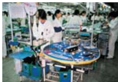
Revolving table production system (Ricoh Component (H.K.) Ltd.)
