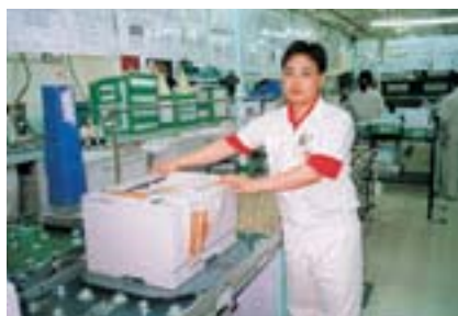
Manually operated production line for printers (RAI)
