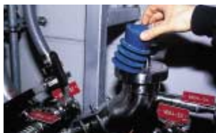
Pipes being cleaned with a pressing ball cleaner and air pressure (Ricoh Industrie France)
