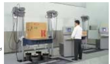
A package's strength is being tested against shock.
