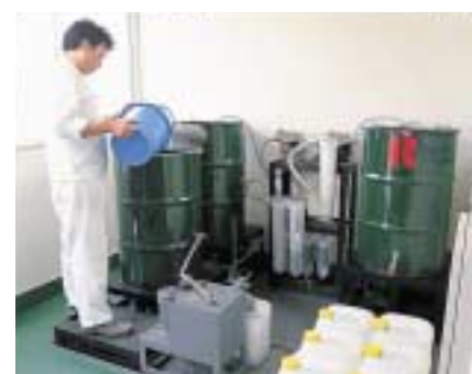
System to reuse lens cutting solution
