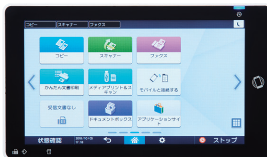
The 10.1-inch MultiLink-Panel, a full-color touch panel, enables users to operate systems intuitively
