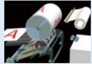
Structural diagram of newly developed one-drum duplex platemaking
