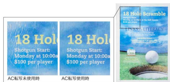
Fig.2 Image samples printed out on the LEATHAC 66 (175 kg) with RICOH Pro C5110S/C5100S. The right is by an ac high field and the left is by simple dc field.
