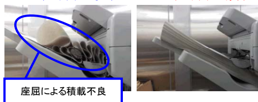
Fig.27 Improvement of stackability of thin paper by the shutter mechanism.
