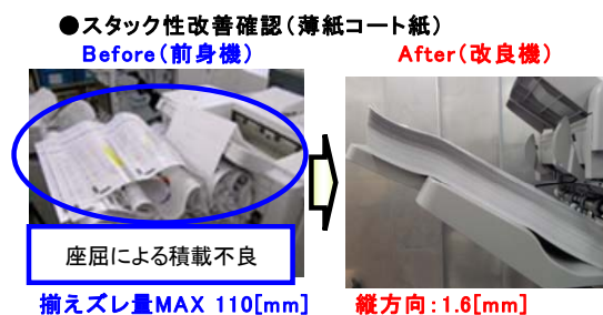
Fig.20 Improvement of stackability for thin and coated paper.
