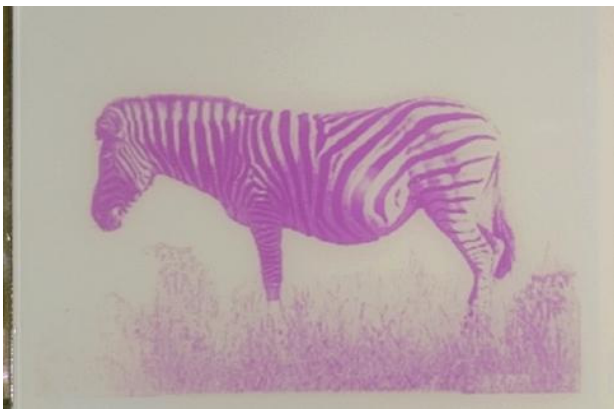
Figure 8. Photograph of AM TFT panel demonstrating mono-color with 64 gray scale.
