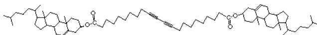
Fig. 5 Chemical structures of medium molecular weight cholesteric liquid crystal for color rewritable recording.
